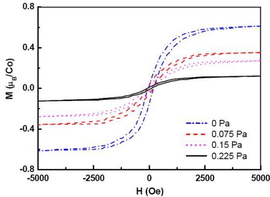
Fig. 2. Magnetization hysteresis curves of 120nm-thick  $\text{Zn}_{0.95}\text{Co}_{0.05}\text{O}$  films deposited under different  $p_{\text{O}_2}$  and  $T_s = 450^\circ\text{C}$  measured at room temperature.
