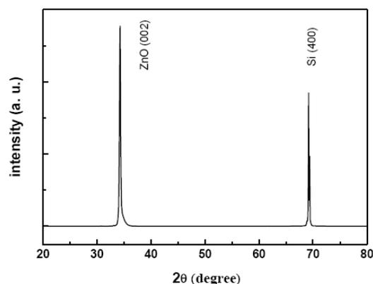
Fig. 1. XRD pattern of a 120nm-thick  $\text{Zn}_{0.95}\text{Co}_{0.05}\text{O}$  film deposited on Si (100) substrate under oxygen partial pressure  $p_{\text{O}_2} = 0.15$  Pa and substrate temperature  $T_s = 450$  °C.
