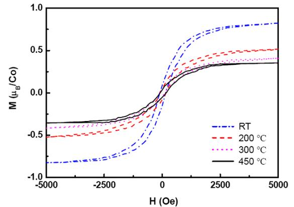
Fig. 4. Magnetization hysteresis curves of 120nm-thick  $\text{Zn}_{0.95}\text{Co}_{0.05}\text{O}$  films deposited under  $p_{\text{O}_2} = 0.075$  Pa and different  $T_s$  measured at room temperature.
