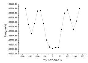
Fig 4. (a) Potential energy profile using B3LYP/6-311++G(d,p) method for the internal rotation around the C7-C6 bond of the title compound.
