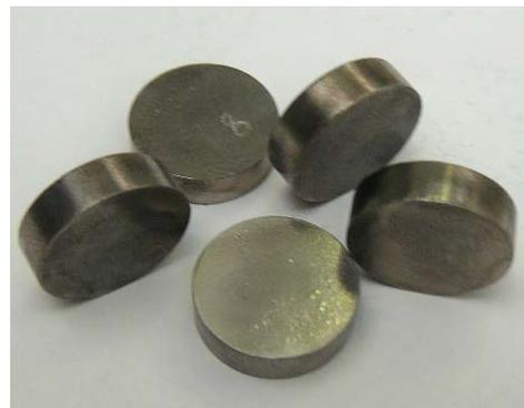
Fig.3. The aspect of the W-Cu (Ni) sintered and infiltrated electrical contacts for vacuum contactors.
