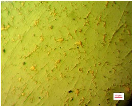
Fig.6. OM image of the W-Cu-Ni sintered and AgCu50 infiltrated electrical contacts (cross section, un-etched state, 200 MPa).
