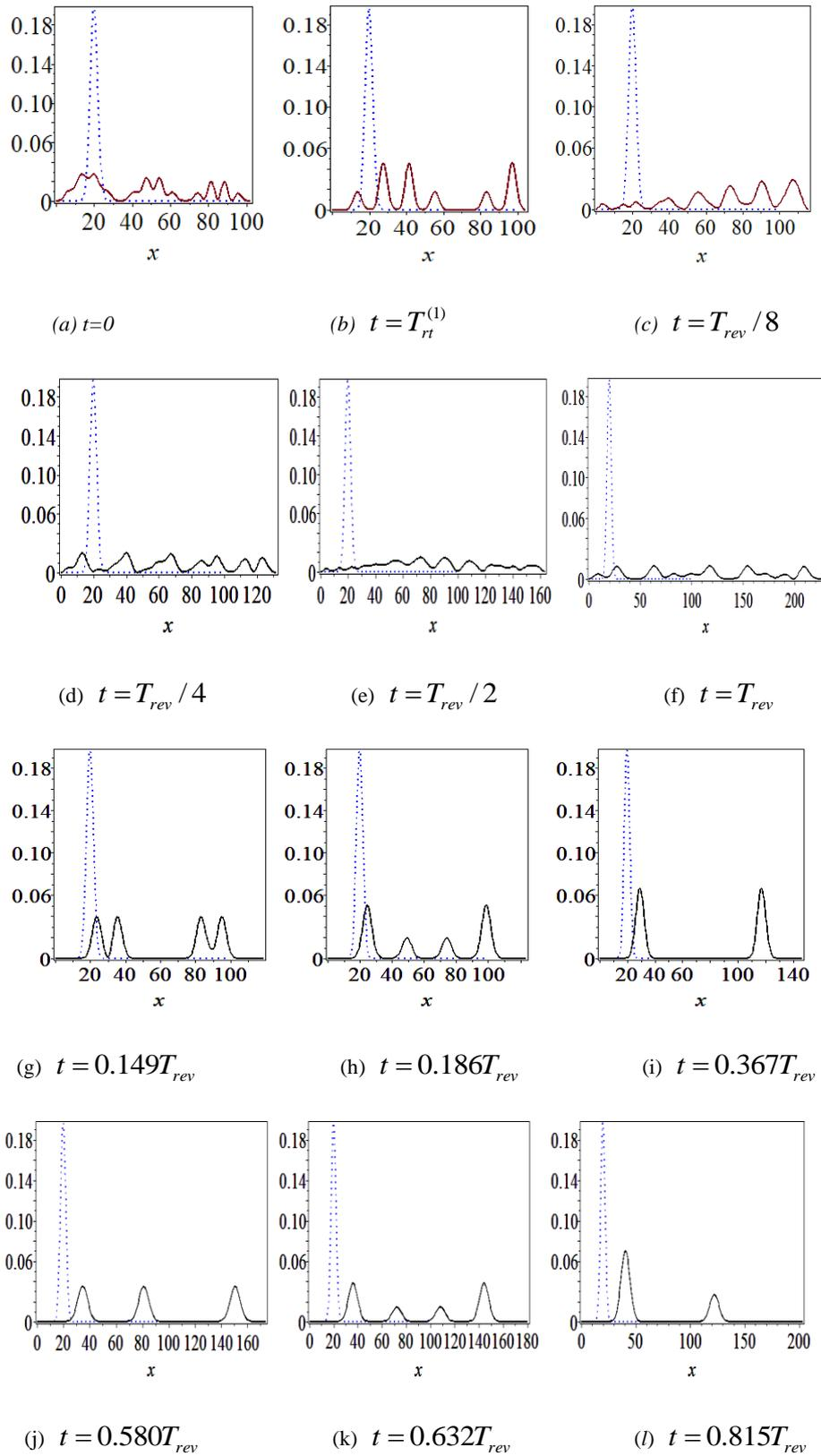
Fig. 4. (color online) The probability density distribution  $|\psi(x,t)|^2$  versus  $x$  in the quantum well with one wall moving fast.
