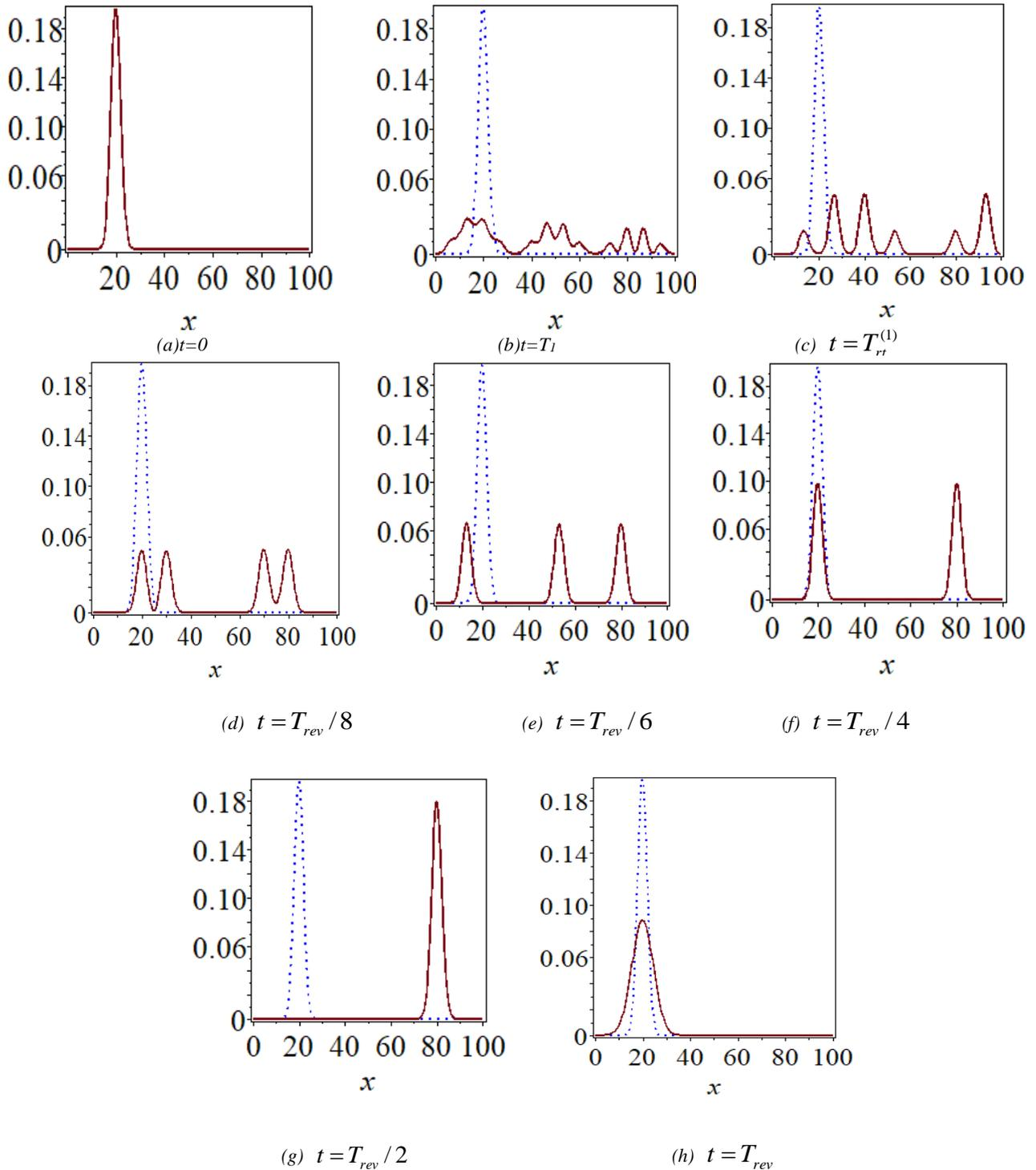
Fig. 3. (color online) The probability density distribution  $|\psi(x,t)|^2$  versus  $x$  in the quantum well with one wall moving very slowly. The moving speed of the wall is  $v=0.00001$ . The times are given in each plot
