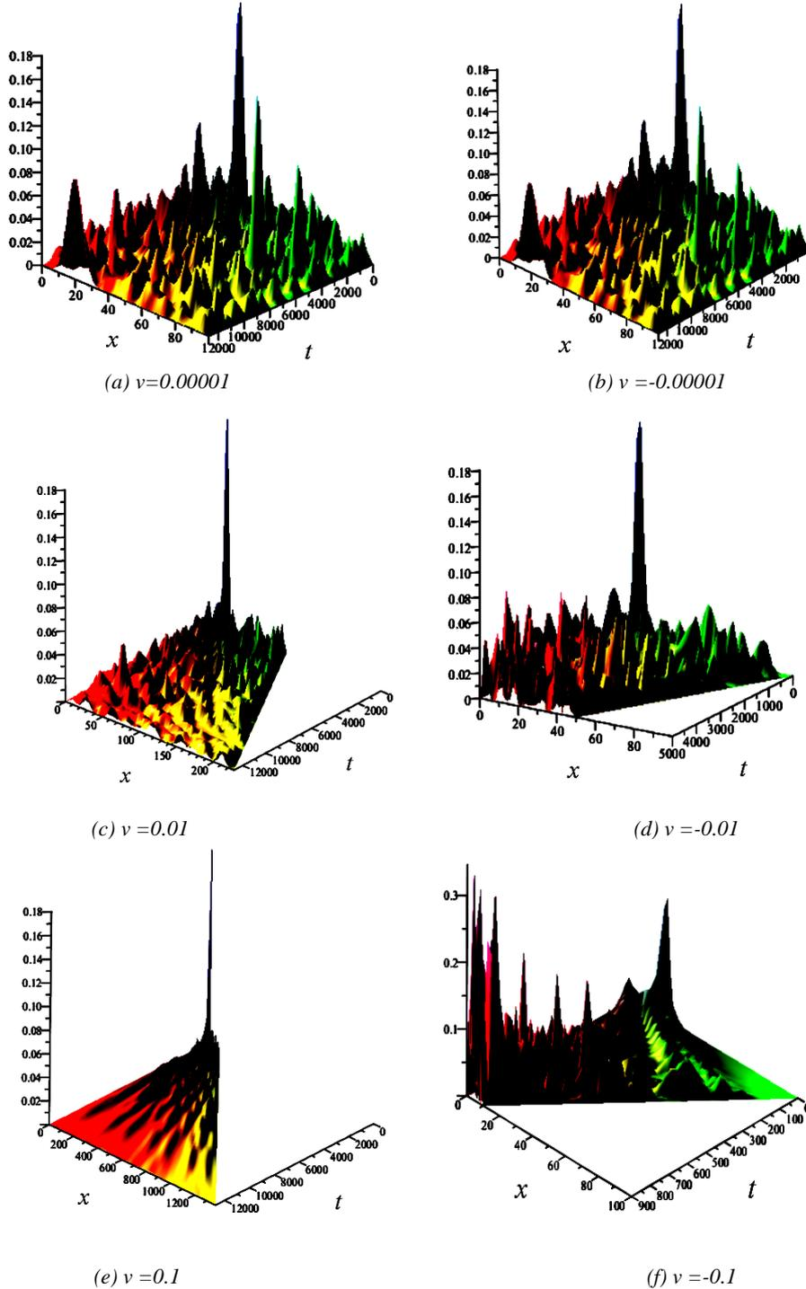
Fig. 1. (color online) The three dimensional probability density  $|\psi(x,t)|^2$  versus  $x$  and  $t$  in the quantum well with one moving wall. The left column corresponds to the case with the wall moving rightward, and the right column is the case with the wall moving leftward. Suppose the initial momentum of the Gaussian wave packet  $P_0=0$ . The moving speed of the wall is given in each plot
